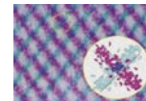
Conventional toner suffers from screen dispersion due to particle size and uneven shape.
